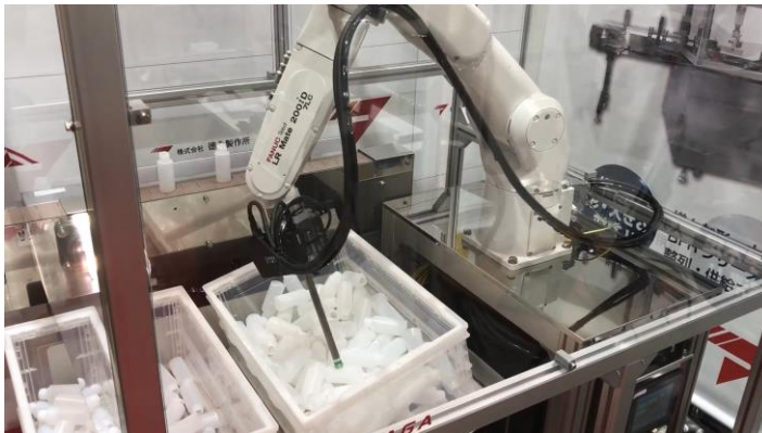
Bulk vacuum picking of (semi-)transparent bottle
