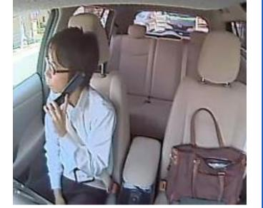
Al controlled analysis of drive recorder video footage of the car interior identifies dangerous behavior such as talking on a mobile phone while driving
